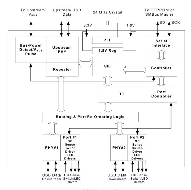
Figure 2.1 USB2512Ai Block Diagram
